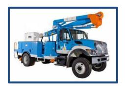
Because of the number of class-6 utility work trucks that operate in the Valley, this project has the potential to demonstrate significant emissions reductions in the on-road vehicle category. The reduced diesel fuel use also reduces greenhouse gas emissions and lowers overall, long-term operating costs for end users.
