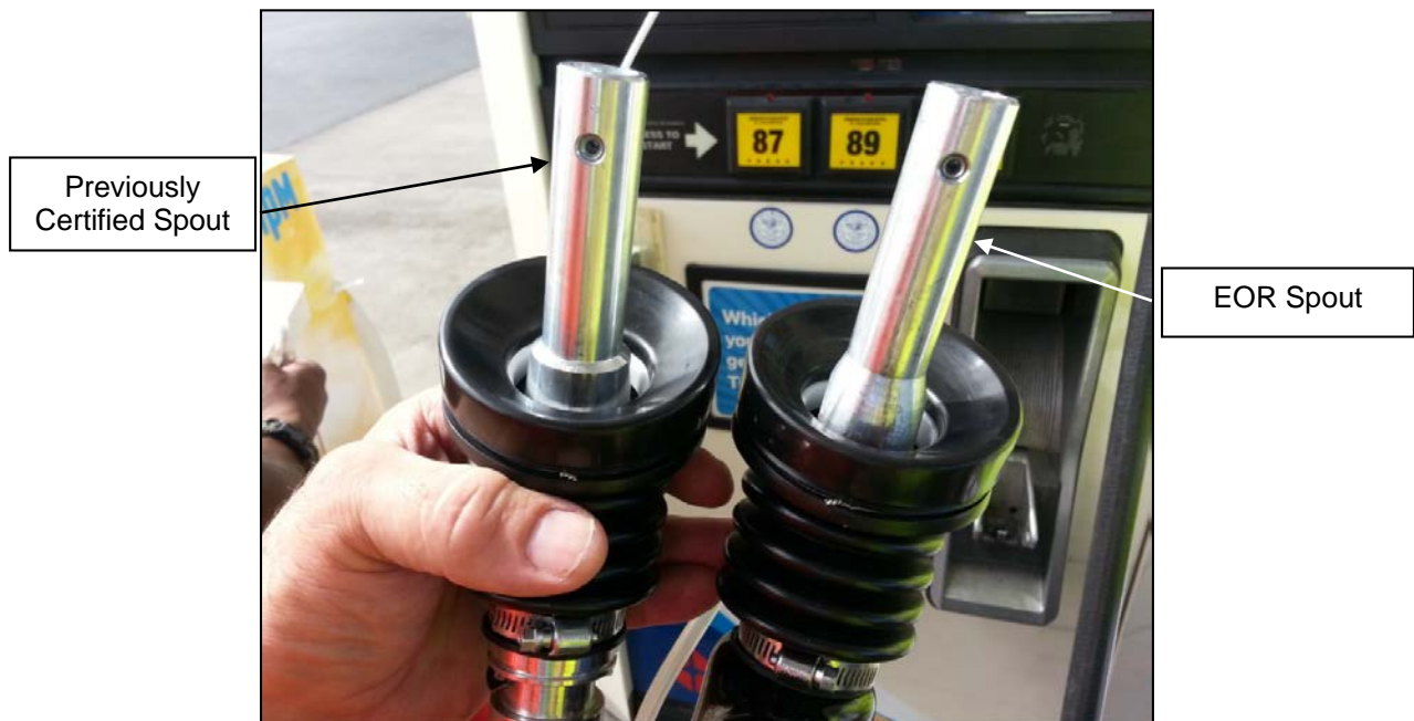
Figure 2: EOR and Previously Certified Spout Assembly (vertical view)
