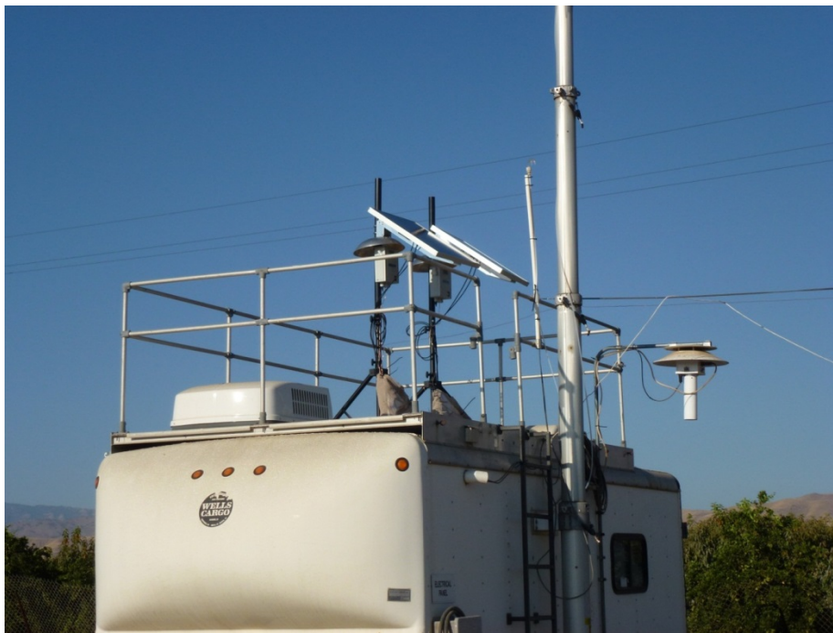
Figure 3-5. Two Aeroqual sensors installed on the roof of the Di Giorgio monitoring shelter.
