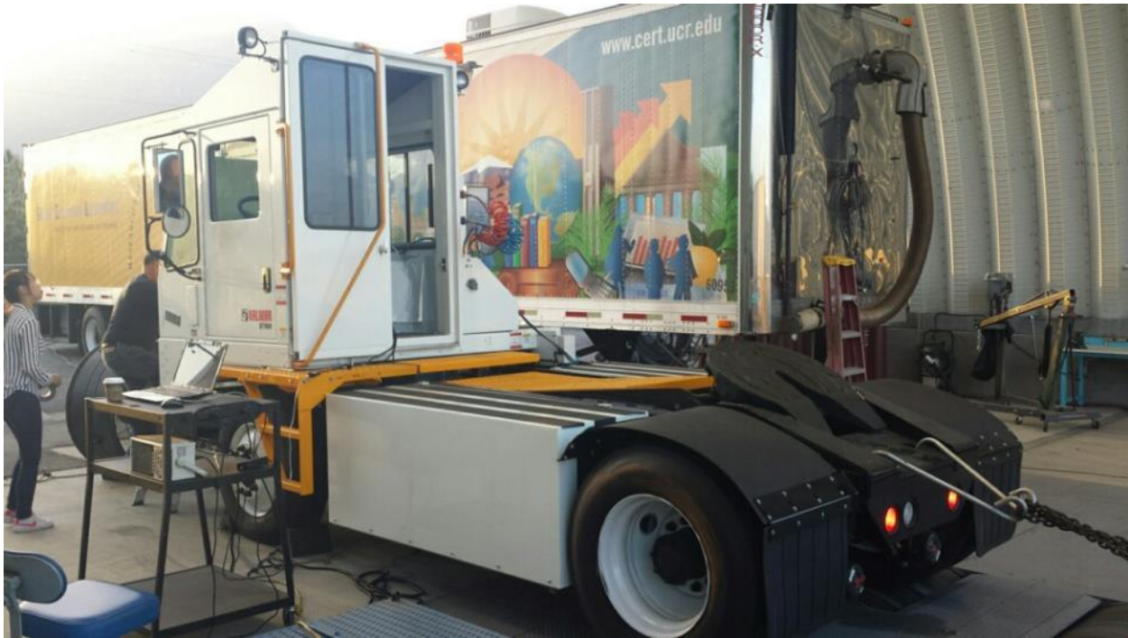
Figure 21. IKEA tractor during dynamometer testing at UC Riverside.
