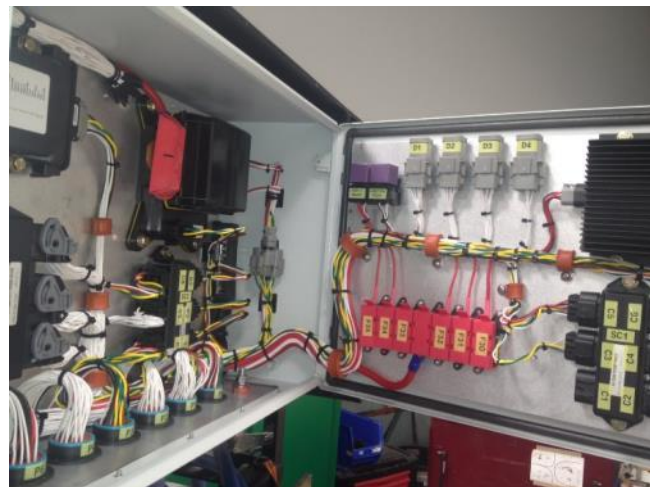
Figure 11. Interior of new CCM as integrated into the IKEA tractor PCAS assembly.
