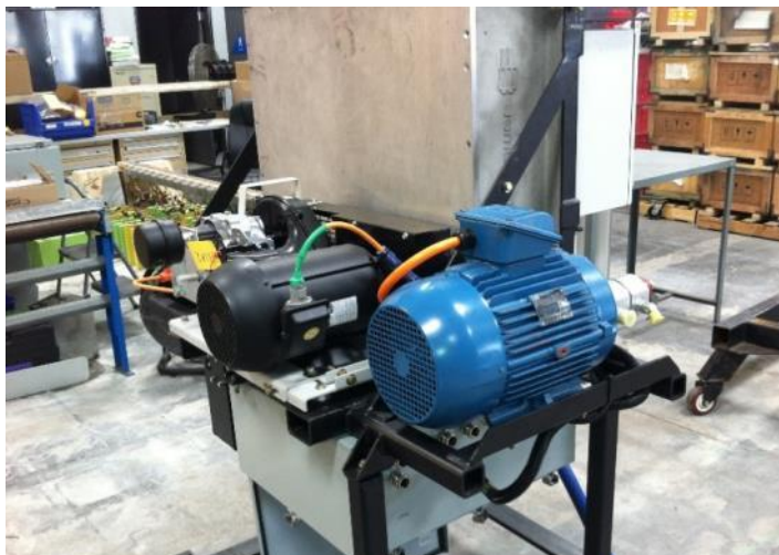
Figure 16. View of the PCAS assembly showing the accessory motors in the foreground.
