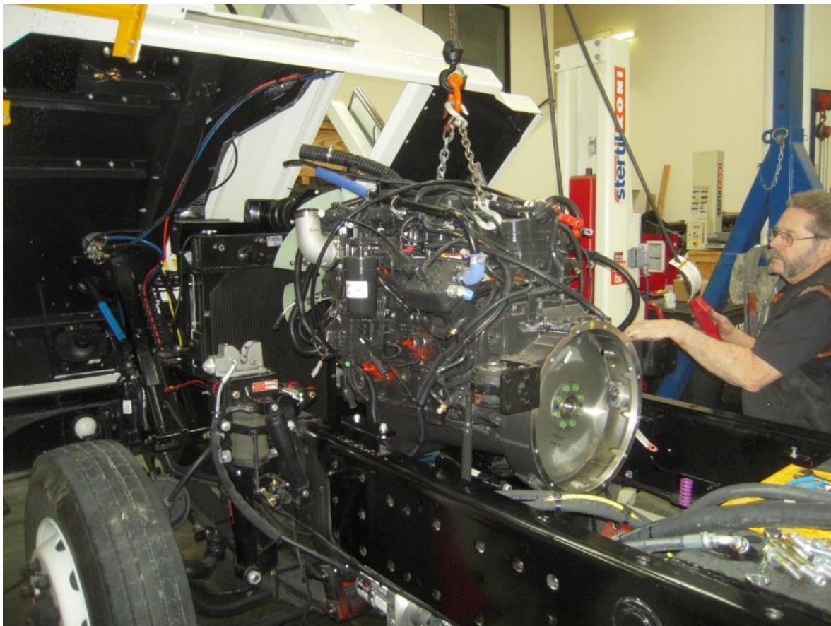
Figure 3. Engine being removed from the tractor.
