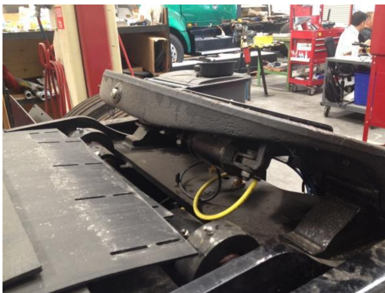
Figure 15. 5th wheel lift on a Kalmar tractor.
