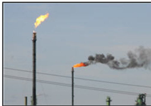
Figure 2 A visual example of complete versus incomplete combustion 3
